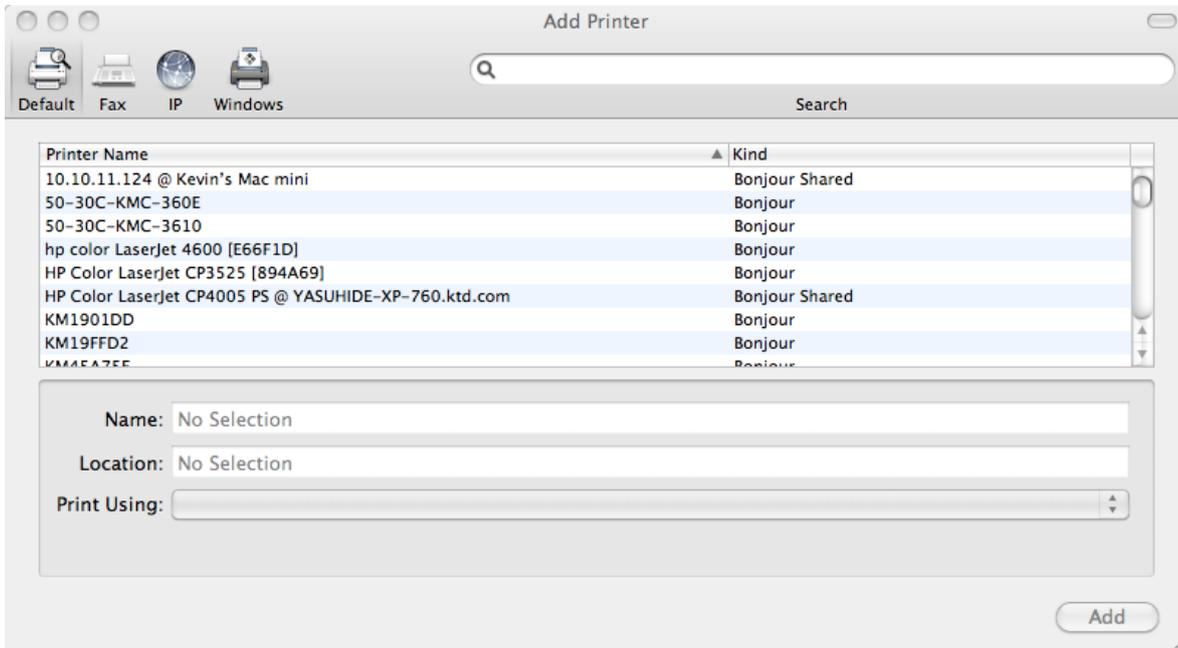
**For better printing support, it is recommended to use Line Printer Daemon (LPD) for the protocol. To add an LPR printer that uses IP, enter the printer's DNS host name or IP address and then select the appropriate model from the Print Using menu. The matching PPD for the printer is automatically selected by the OS.**
