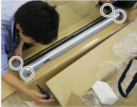
Remove the transfer/detach corotron from the box, and remove the metal plates with two screws each attached to the transfer/detach corotron's right and left.
