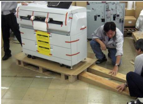
Set ramps as the left photo shows. Then slowly move the Printer over the ramps.
