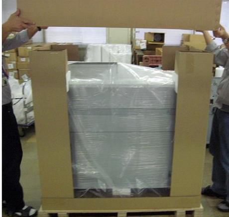
Raise and remove the top panel and sleeve.
