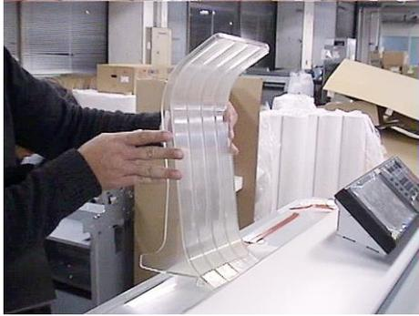
Attach the two original output guides.
