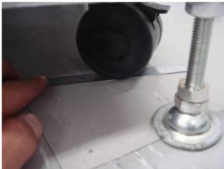
Turn the nuts to lower the four adjustable leveling feet until the four casters are about 1 mm off the floor.
