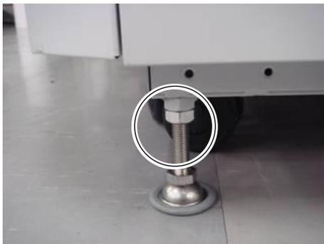
After adjusting all four positions, tighten each nut to secure the adjustable leveling feet.
