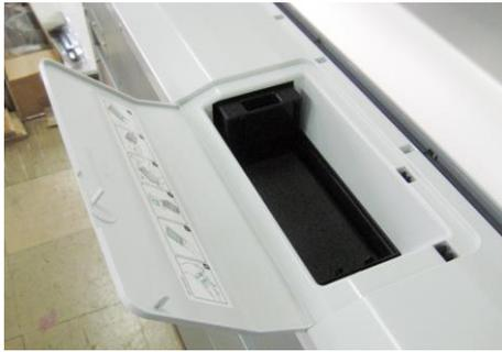
Open the toner cover and remove the dummy toner cartridge.
