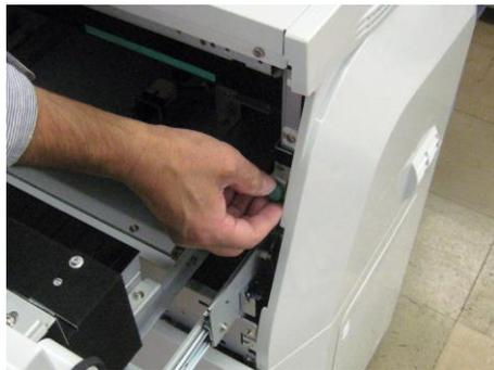
Turn the external knobs to open the process cartridge drawer.
