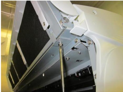
Remove the two brackets on the right and left keeping the document table at an angle.
