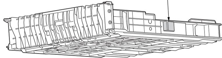
\*Leave it for about 30minutes (drying time) after painting HANARL SF-133, and then Assemble the Cassette-Assy to printer.
