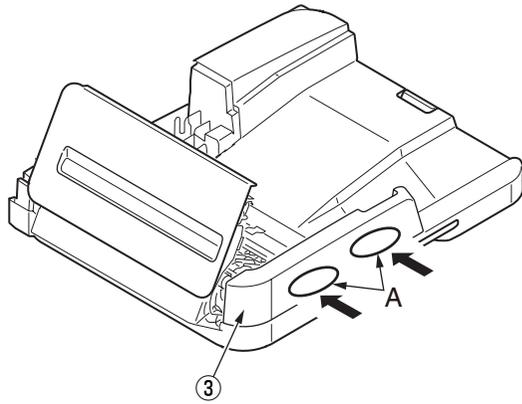
(6) Remove the cover-ADF-F (3) in the direction of the arrow.
