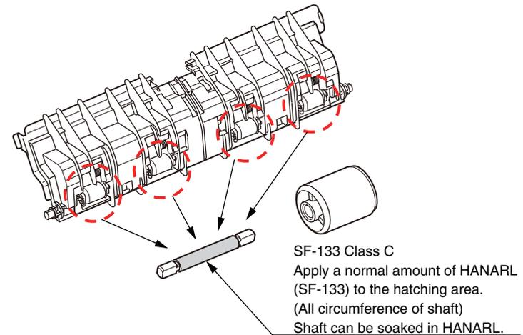
※ Leave it for about 3minutes (drying time) after painting HANARL SF-133, and then assemble the roller.
