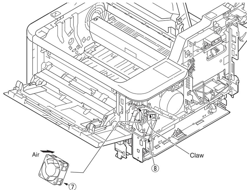
(7) Remove three screws (Silver) ⑨ to detach Duct Fan Power ⑧ .
