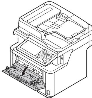
(3) Close the MPT gently to a position where the left and right tabs fit the arm grooves.
