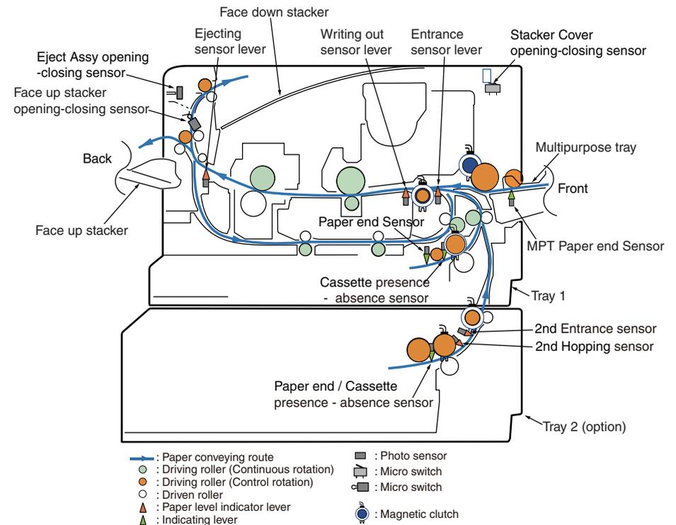
Figure 3-1 The sectional view of only printer
