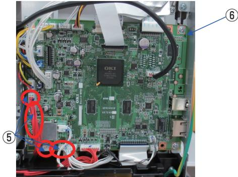
(5) Remove the PWR unit-ACDC Switch. (Refer to 4.2.4).
