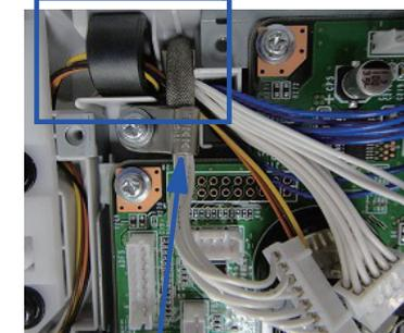
The cable with the shield should be in the highest position.
