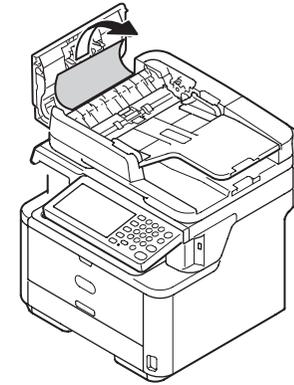
If the edge of the document can be seen under the paper guide ①, lift the paper guide and then pull out the document.
