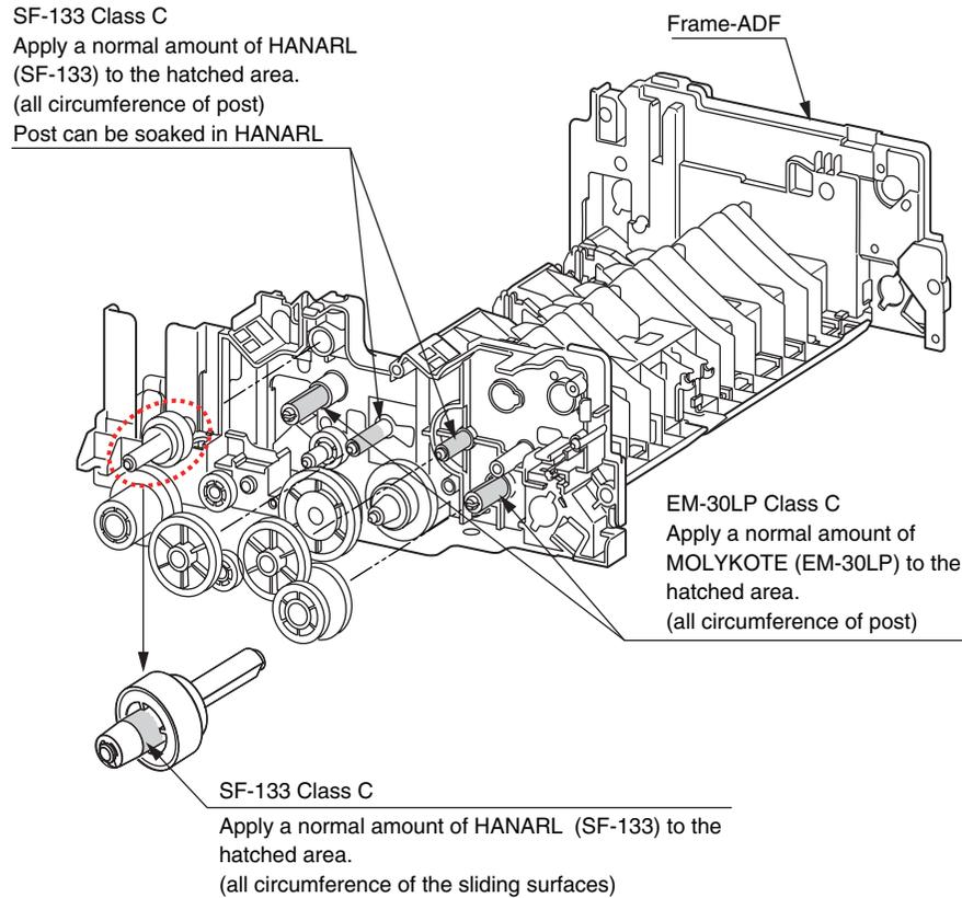
※ Leave it for about 3minutes (drying time ) after painting HANARL SF-133, and then assemble the ADF-Assy.
