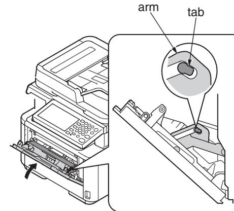
(4) Separate the tabs on the roller guide from the left and right arms by opening the arms outside.
