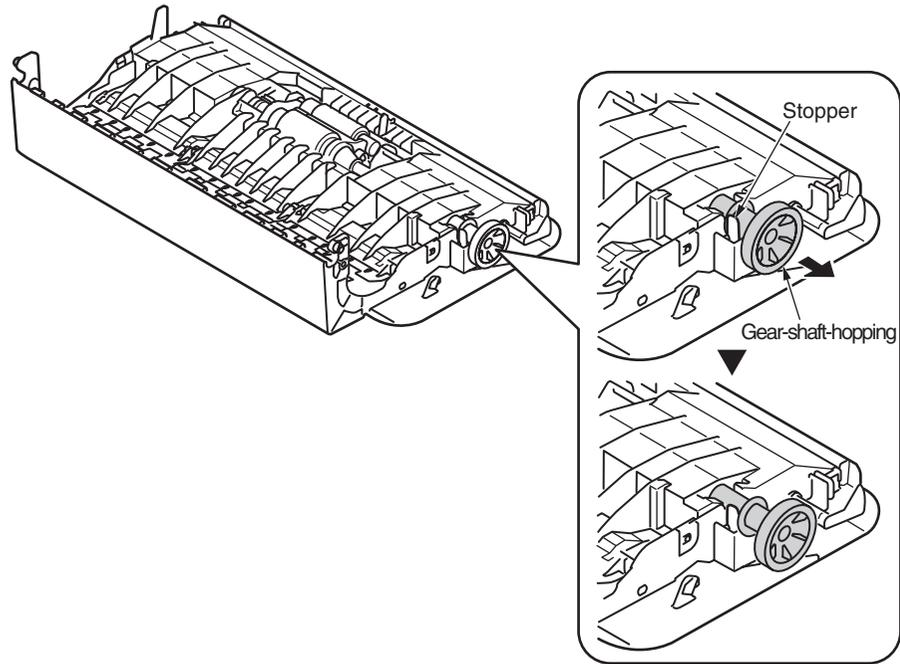
(2) Remove the Frame-assy-hopping-ADF ① and the Stopper-Assy-Gate ② .
