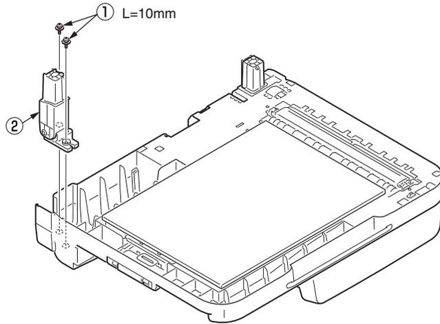
(2) Remove two screws (L=10mm) ④ and remove the hinge-Assy-L ⑤ .
