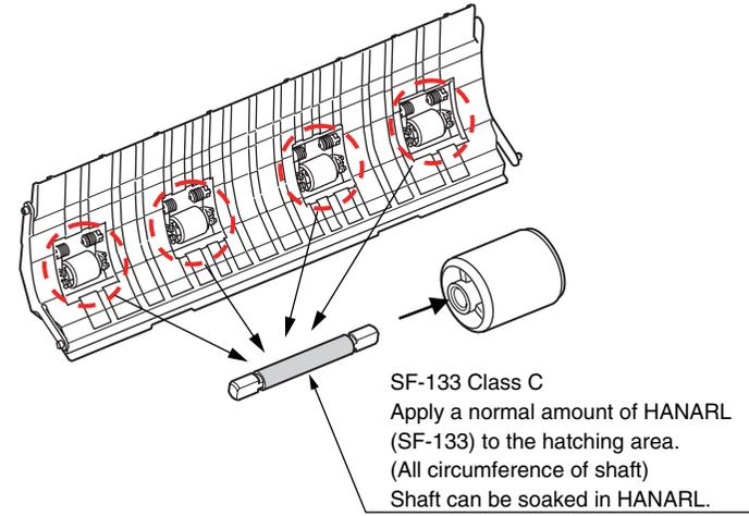
※ Leave it for about 3minutes (drying time) after painting HANARL SF-133, and then assemble the roller.
