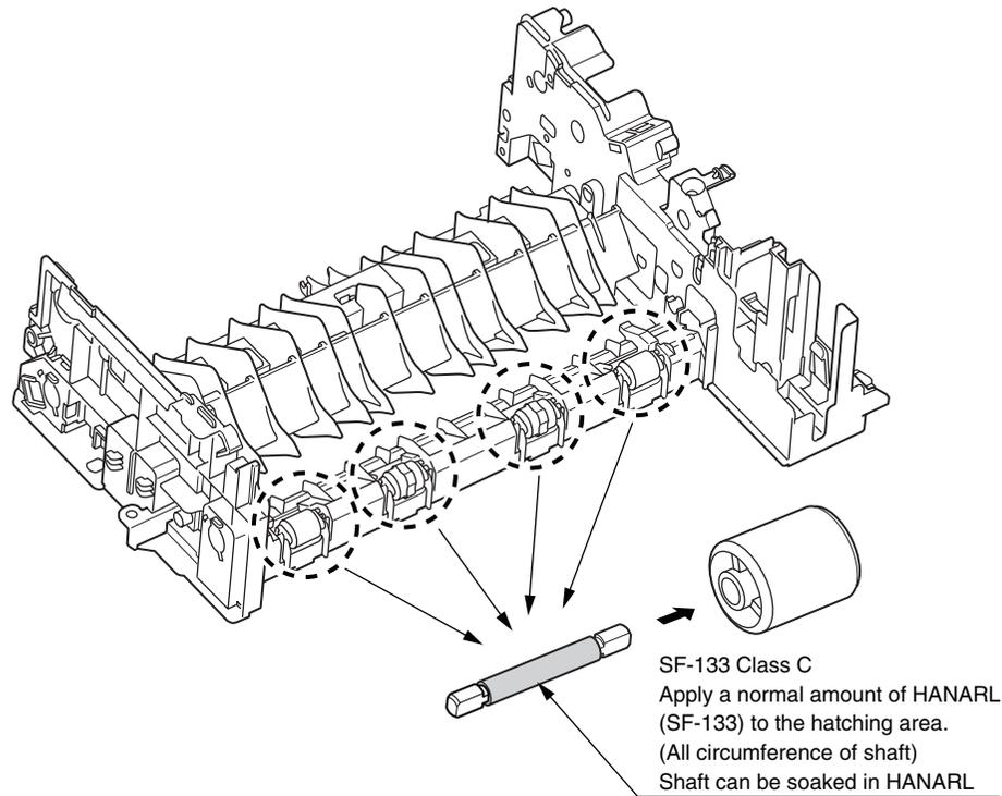
※ Leave it for about 3minutes (drying time) after painting HANARL SF-133, and then assemble the roller.
