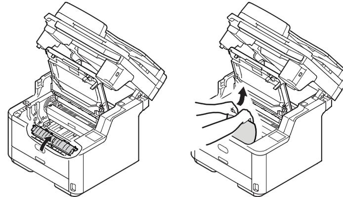
If neither the top or bottom end of paper is visible, move the jammed paper in the arrow direction as shown. Hold the top end of paper by your hands and carefully pull out the paper.
