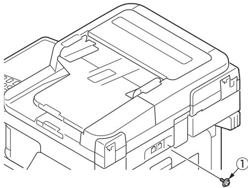
(2) Remove four screws (black-colored, L=10mm) ② to remove the Cover Bottom ③ .
