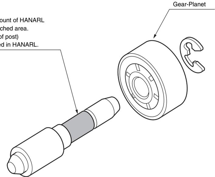
※ Leave it for about 3minutes (drying time) after painting HANARL SF-133, and then assemble the Gear-Idle-Assy.
