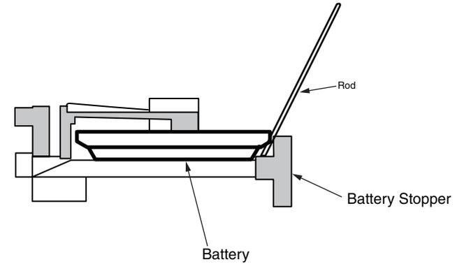
Raise the battery up so that it is put on the battery stopper, and remove it.
