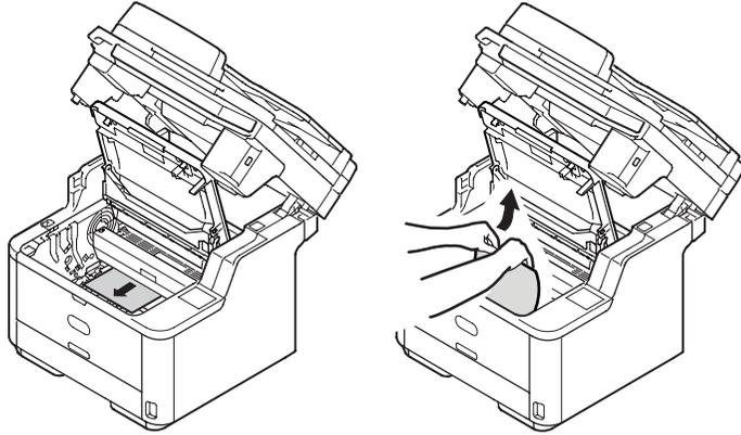
If the bottom end of paper is visible, hold the paper by your hands and carefully pull out the paper.
