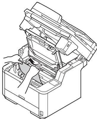
• If the bottom end of paper is not visible but its top end is visible at the paper discharge unit, hold the top end of paper and pull out the paper carefully. If you cannot remove the paper by following Steps (A)1 and (A)2, pull out the paper by following Steps (B).
