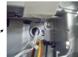
Clamp together the screw and the FG-Film.
