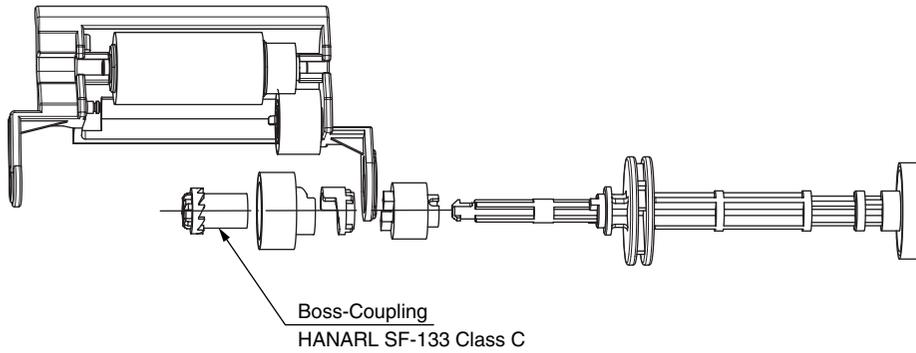
Leave it for about 30 minutes (drying time) after painting HANARL SF-133, and then assemble the Boss-Coupling.
