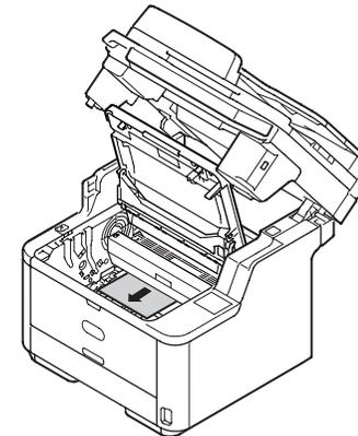
If the bottom end of paper is visible, hold the paper by your hands and carefully pull out the paper.
