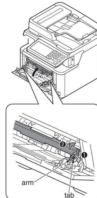
(5) Raise the roller guide until it comes in contact with the MFP.
