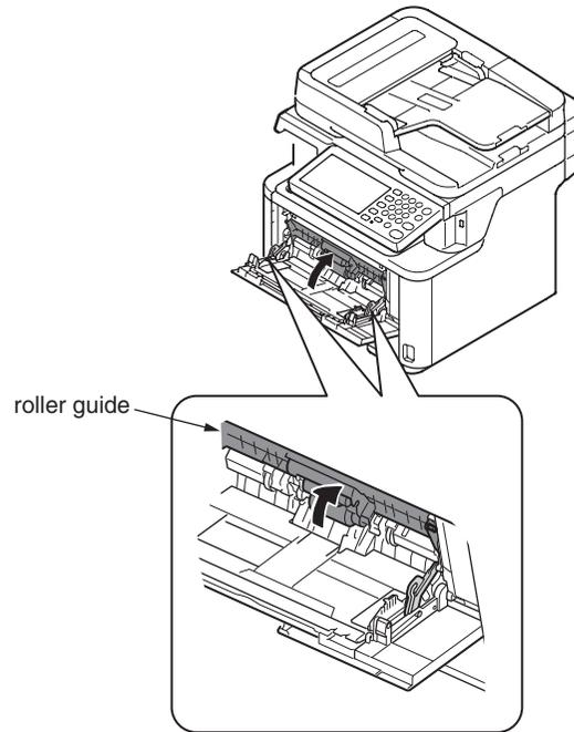
(6) Wipe the two feed rollers with a tightly wrung cloth soaked in water through the opening for MPT.
