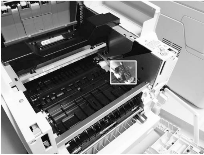
Drum & Toner Contact Location within the printer
