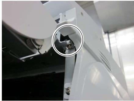
With the screws and the grooves hooked, lift the front edge of the document table up until it is perpendicular to the surface attached. Keep the document table in that position.
