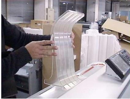
Attach the two original output guides.
