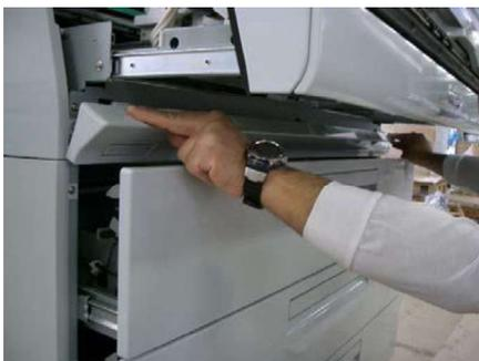
Insert the bottom side tabs into the printer. While pressing the top side tabs from above, attach the electrical box access cover.
