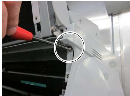
Tighten the right and left screws. However, to allow the document table to be moved to the right and left, loosen the two screws one turn from the fully tighten position.
