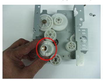
7.5 - Remove 2 bushing and one E-clip from the ends of the shaft.
