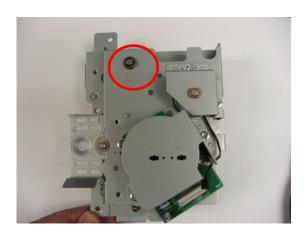
7.2 - Turn the drive unit over and remove the 2 screws shown here.
