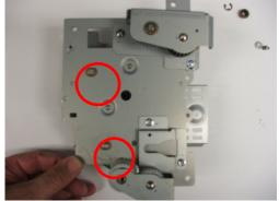
7.12 - Reinstall the 2 screws holding the two halves of the drive unit together.
