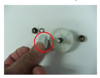
7.7 - Confirm the new replacement gear by locating the Black dot on the back side of the gear.
