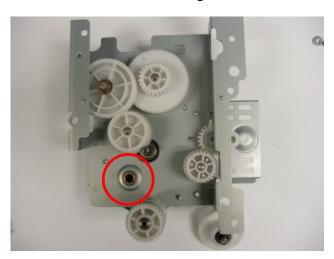
7.10 - Reinstall the gear into the drive assembly
