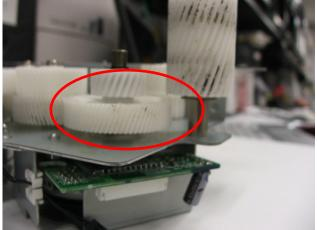
7.11 – Reinstall the bushing on the shaft with keyed side facing up and replace top half of the drive assembly. Be careful to align both bushings with keyed holes.
