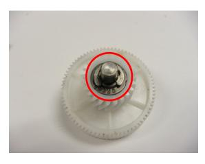
7.9 - Insert the bushing into the hole in drive unit frame.
