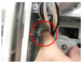
6.4 - Remove 4 screws and carefully remove the fuser drive unit by lifting up and rotating.
