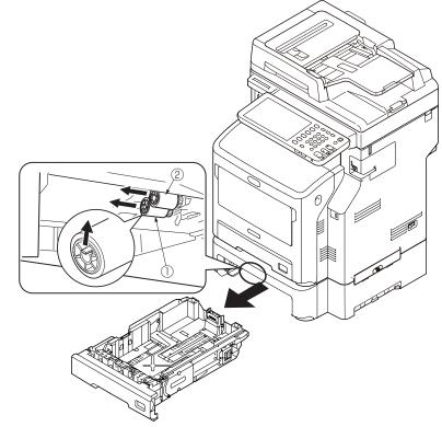
(3) Set the new roller (with gear)  $\bigcirc$  to the shaft.
