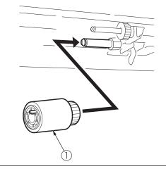
(4) Set the new roller (without gear) (2) to the shaft.
