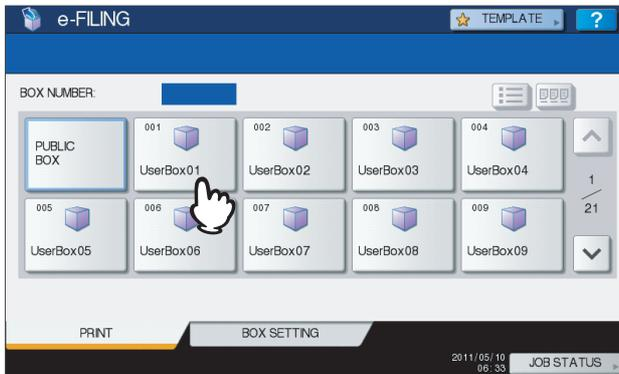
Press or to switch the pages. You can also specify the box number (3-digit) using the digital keys.
